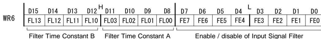
D7~0 FE7~0 For each input signals as shown in the table below, it can set whether the IC built-in filter function is enabled or the signal is passed through.
