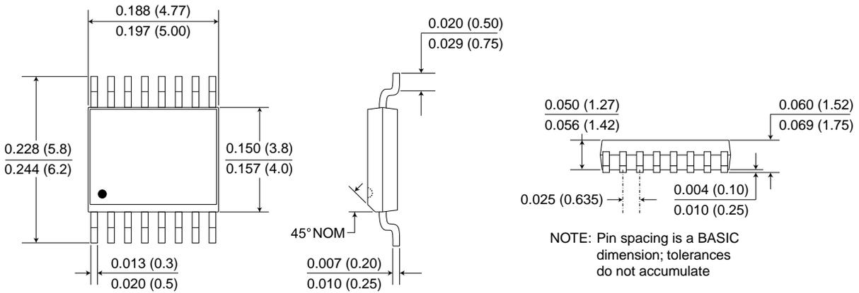
**0.15" 16-pin SOIC Package (-3 suffix)**
