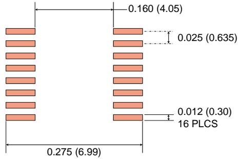
**0.15" 16-pin SOIC Pad Layout**
