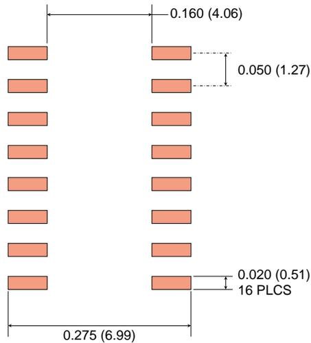
**0.3" 16-pin SOIC Pad Layout**
